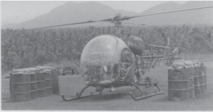
One of the helicopters chief assests was the ability to operate from forward bases. This OH-13 sits between makeshift revetments of old 55 gallon drums and sandbags in the An Lao valley during the fall of 1967. The ship is from the 1st Squadron, 9th Cavalry Regiment of the 1st Cavalry Division. (US Army)
