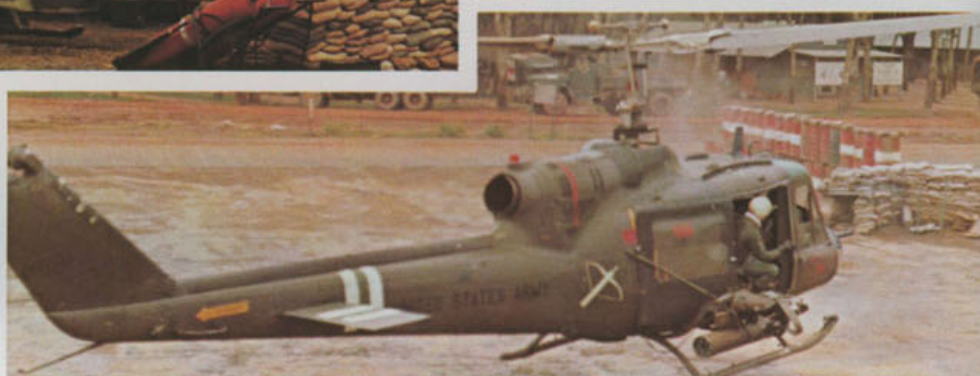
(Above Right) In an attempt to provide Huey door gunners with more firepower a pair of M-60s were sometimes mounted on a modified gun pedestal. These M-60s have been modified from the standard infantry weapon.
