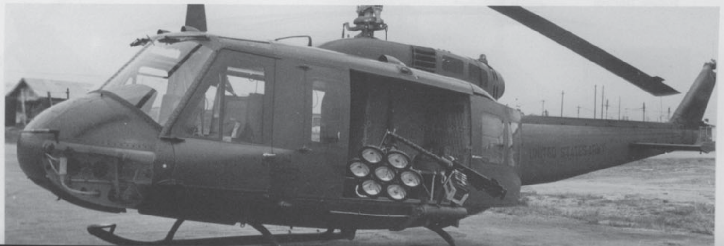
This UH-1D 'lightning bug' carries a hand fired .50 caliber machine gun for surpression fire. Although such heavy weapons were not normally fitted to the Huey, various experiments and field modifications were tried throughout the war to increase the helicopter's offensive firepower. (US Army)
