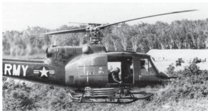
A UH-1A makes a practice run at a firing range outside of Saigon. Notice how the crew chief is holding the cocking lever. These first gunships did not have side mounts for additional machine guns as did later versions of the Huey series. (Bell)
