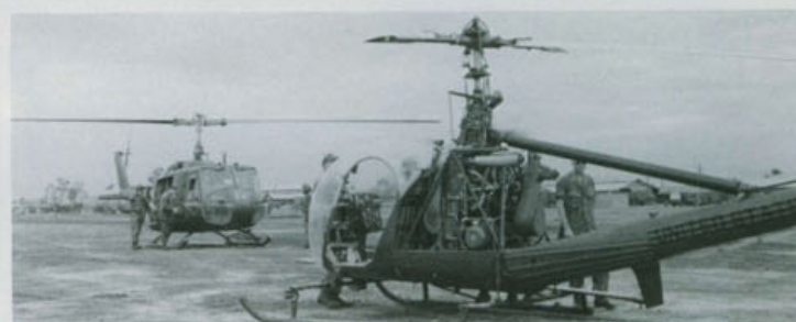
An OH-23 and UH-1D sit on the landing pad at Di An while the crews try to repair the light observation helicopter for a flight back to the base at Ben Cat. Visibility from the OH-23's bubble canopy was excellent, although when it hovered the crew sweltered under the direct rays of the sun as there was little air movement in the cockpit. (US Army)
